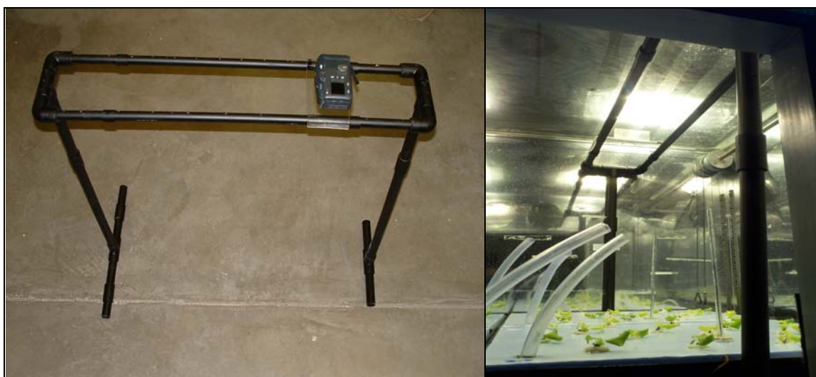
Figure 1. Frame to hold the digital camera (left) and the frame position inside the growth chamber (right).
